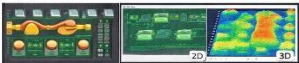
Detected bridging defect by SPI system
