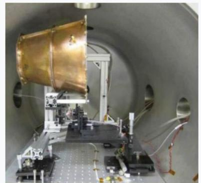
EmDrive built by NASA Eagleworks laboratory during their 2013–2014 experiments
